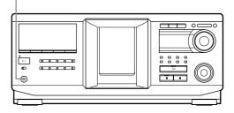
**1** Connect a keyboard to the keyboard jack on the front panel of the player.
